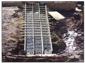
Figure 1. Rectangular Channel Setup
